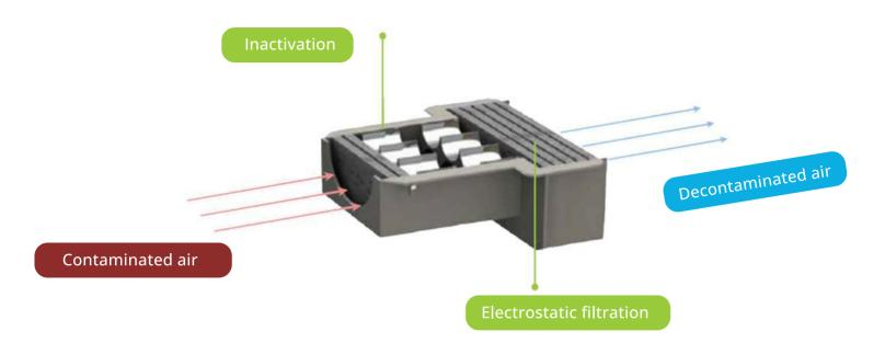
The airflow passes through constant electric fields created by crosswise air-permeable electrodes consisting of high porosity conductive plates made of foamed metal. The electrodes are connected with a high-voltage power supply source to have alternating polarity. In twin-section charging chambers, the surface and intracellular and molecular structures are recharged many times, which inactivates (destroys) bacteria and viruses, and retains the destroyed biomass in the electrostatic precipitator.
